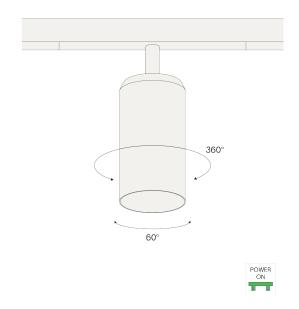
Slide the luminaire in the prado 48V track make sure to use a prado 48V LED-driver.
