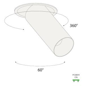
Twist the luminaire as desired.
