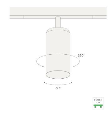
Slide the luminaire in the prado 48V track make sure to use a prado 48V LED-driver.
