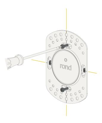
Level kit, gently screw with appropriate stainless steel screws.
