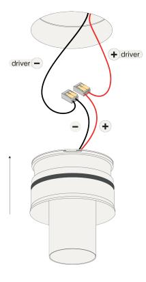
Connect the wires with the connectors for serial connection, respect polarity combine with a prado LED-driver.
