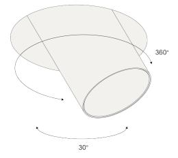
Twist the luminaire as desired.
