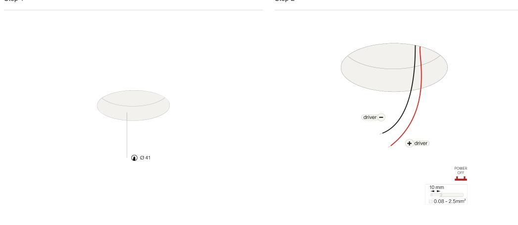
Cut a round hole (Ø41). Consult the chosen luminaire tech specs for required height and free air dimensions.
