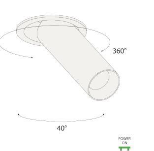
Twist the luminaire as desired.
