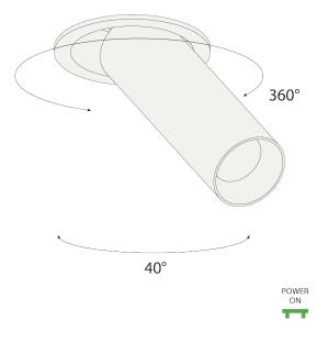
Twist the luminaire as desired.
