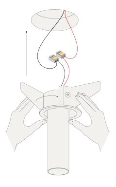
Connect the wires with wago connectors for serial connection, respect polarity combine with a prado LED-driver.
