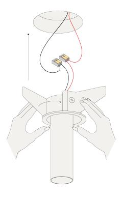
Connect the wires with wago connectors for serial connection, respect polarity combine with a prado LED-driver.
