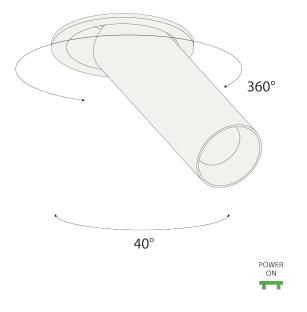
Twist the luminaire as desired.
