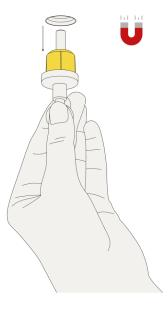
Twist the yellow plaster lid with a screwdriver before removing it with a magnet.
