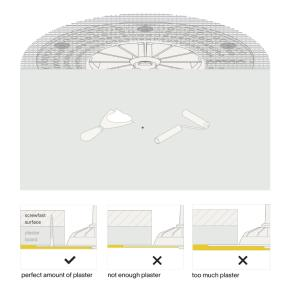
Insert the plaster ring and securely fasten it with glue or the appropriate screws on a screwfast surface. The attachment must be able to obtain a static load of 5 kg. It's the installers responsability to ensure optimal attachment. We advise to test the electrical connection before starting to plaster.
