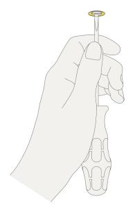
Carefully remove excess plaster to access the screw. You can easily locate the jack kit by using a magnet.
