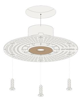
Cut a round hole ( $\emptyset$  68). Consult the chosen luminaire tech specs for required height and free air dimensions.
