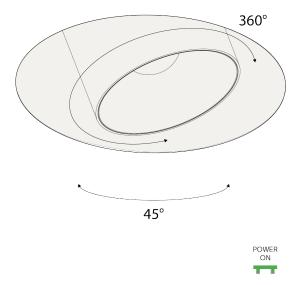
Twist the luminaire as desired.
