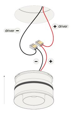
Connect the wires with the included connectors for serial connection, respect polarity combine with a prado LED-driver.
