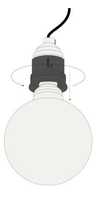
Screw the light bulb into the prado invisible E27 socket.
