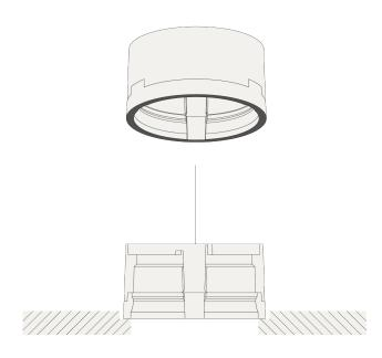
Mill a hole with the above dimensions in a wooden base (not supplied) (maximal fabric thickness : 1.2mm).
