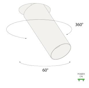
Insert the luminaire into the ceiling until it "clicks". Push the luminaire a little further and twist it to lock it. Gently pull the luminaire down again. Now it's locked.
