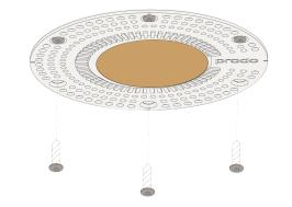
Cut a round hole ( $\emptyset$  68 - depth depends on fixture type).
