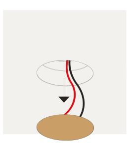
Excercise caution while plasering, do not damage the ring. Keep the plaster lid inside the plaster ring while plastering. Use a fiberglass mesh tape to ensure optimal plaster adhesion. Make sure not to touch the edge of the ring when sanding.
