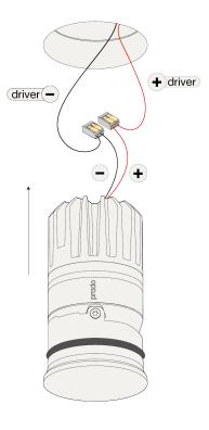
Connect the wires with the included connectors for serial connection, respect polarity combine with a prado LED-driver.
