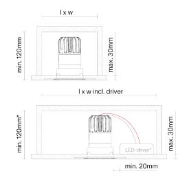
\*make sure the selected driver fits thu the hole and inside the free air dimensions
