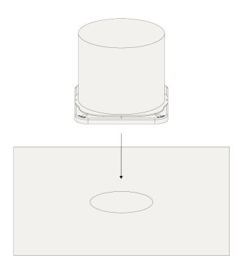
If the finish material thickness is not 19mm, machine down or add (wooden) plate to achieve the correct total depth (19mm).
