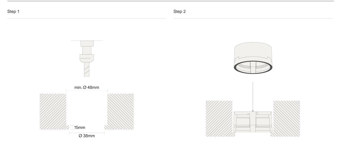
Mill a round hole with the above dimensions. Consult the chosen luminaire tech specs for required height and free air dimensions.
