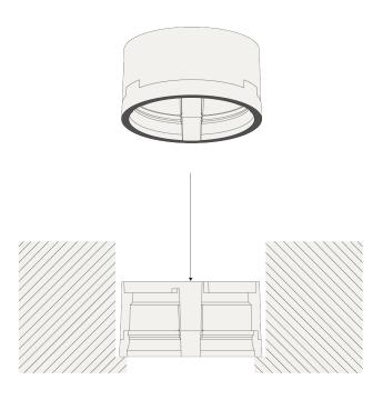
Mill a round hole with the above dimensions. Consult the chosen luminaire tech specs for required height and free air dimensions.
