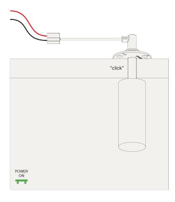
Make the electrical connection and test it before closing the ceiling. Do not plug or unplug the fixure while power is on.
