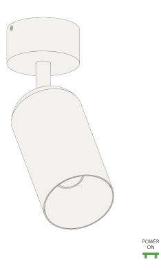
Twist the luminaire clockwize and fasten the screw to lock the luminaire.
