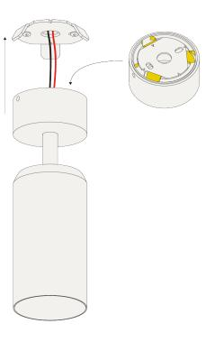
Connect the wires with the wago connectors for serial connection, respect polarity combine with a prado LED-driver.
