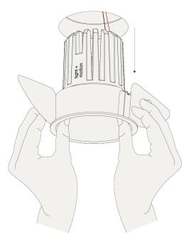
For both maintenance and the adjustment of settings, the luminaire can be removed from the ceiling.
