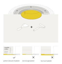
Insert the plaster ring and securely fasten it with glue or the appropriate screws on a screwfast surface. The attachment must be able to obtain a static load of 5 kg. It's the installers responsability to ensure optimal attachment.
