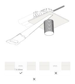
Connect a Ø16 preflex and the ventilation duct with the prado connector. Make sure to add at least 300mm of wire into the ventilation duct. Driver must be placed remotely to remain accessible.
